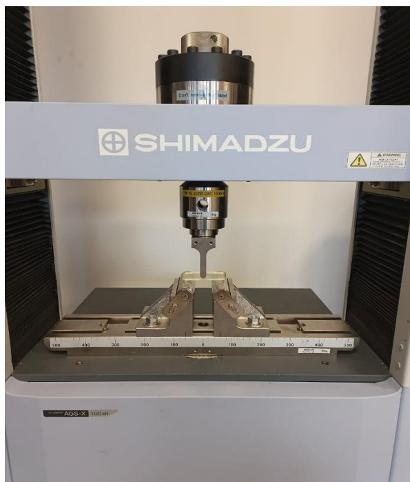
Figure 2. Three-Point Bending Test Specimen and Test Setup
