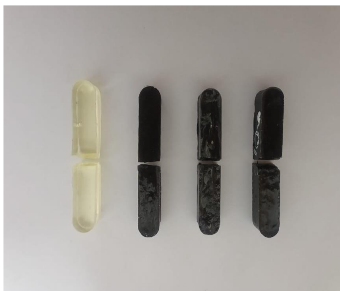
Figure 3. Epoxy/Matrix Materials with 0%, 0.5%, 1.5%, and 3% Carbon Fiber Reinforcement After Three-Point Bending Test
