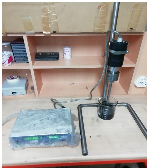
Figure 3. Sonicator mixing process of CNF and Epoxy
