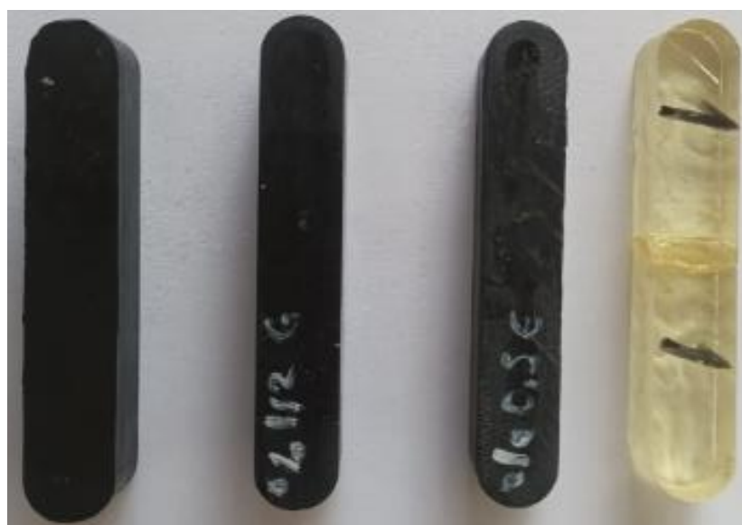
Figure 5. CNF filled and unfilled epoxy composites prepared for testing
