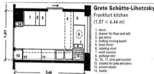
Figure 6. Detailed drawing of Frankfurt kitchen exploring intelligent design (source:Karel Teige)
