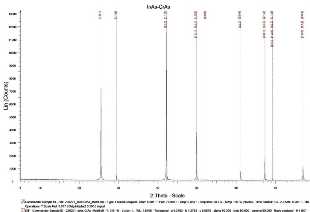
Fig.1. X-ray spectrum of InAs-CrAs eutectic composite.
