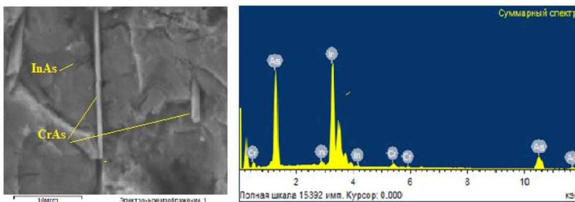
Fig.3. X-ray spectra of InAs-CrAs obtained with SEM-EDX from the needle and matrix phases along the lateral directions of the specimens
